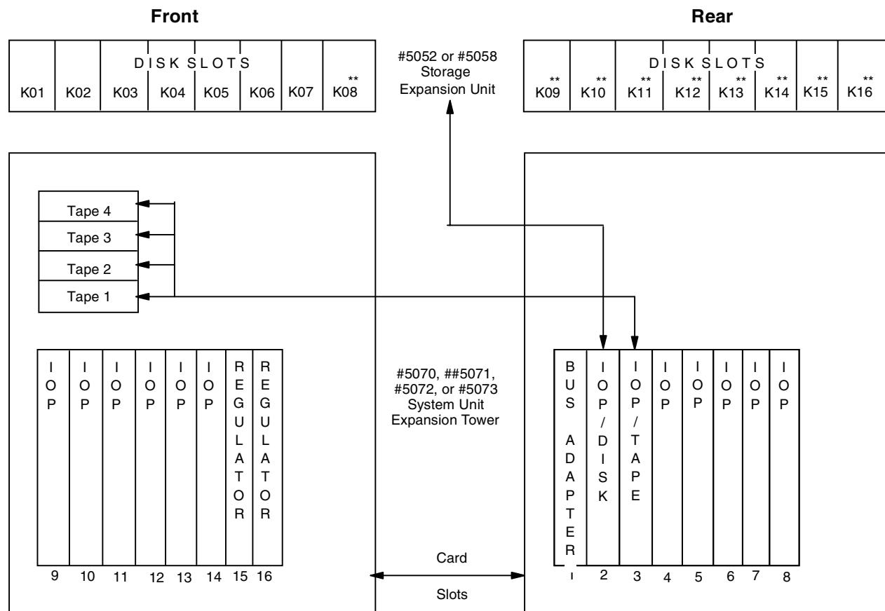
\*\* One-byte disks cannot be installed in disk slots K08 through K16.
