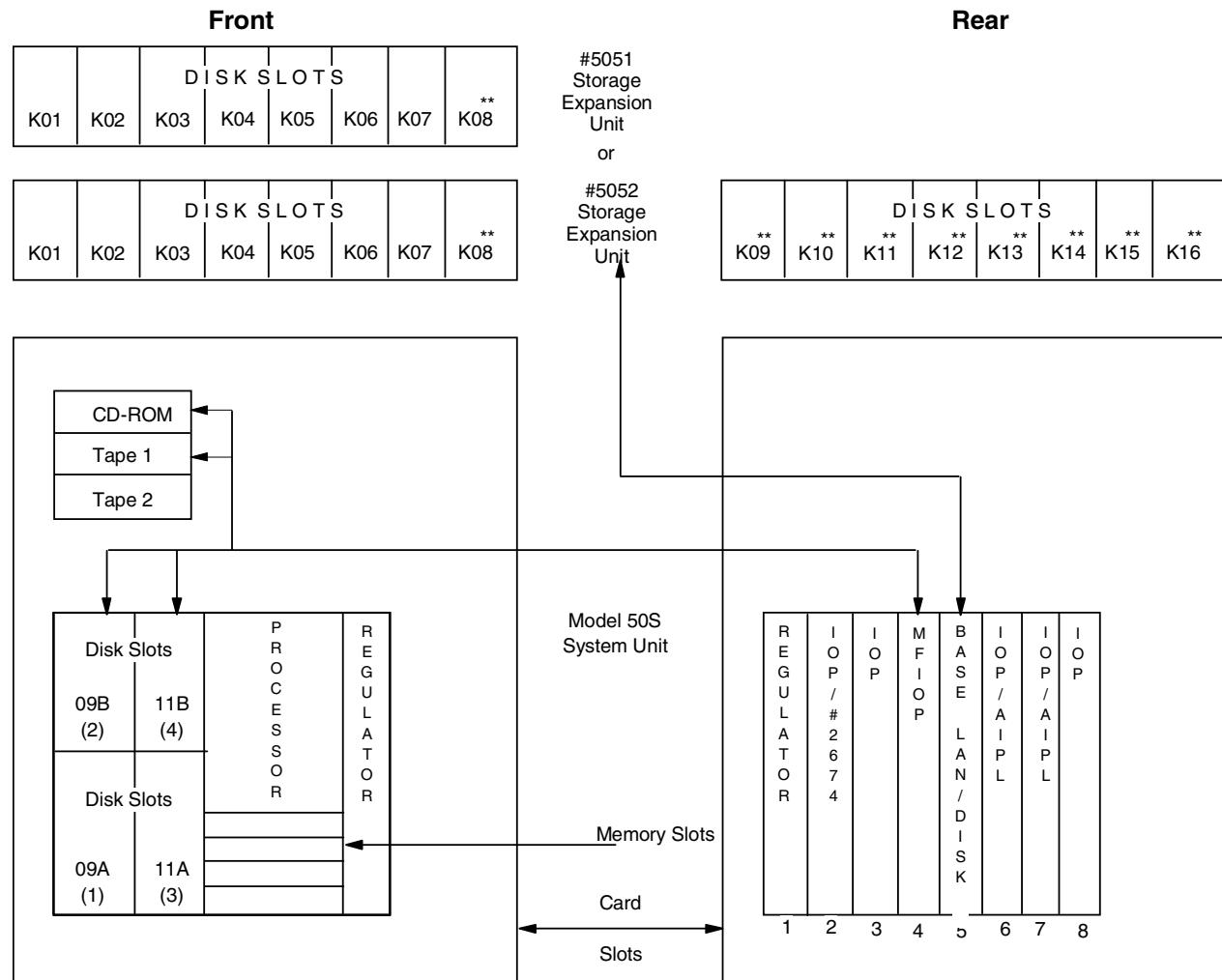
\*\* One-byte DASD cannot be installed in disk slots 8 through 16.
